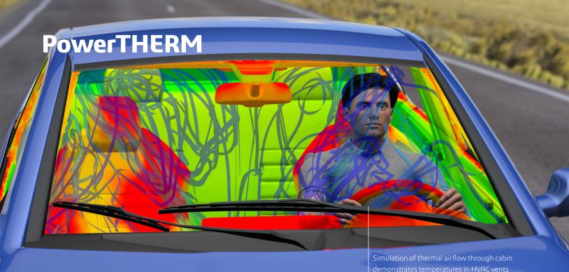
demonstrates temperatures in HVAC vents and on human model using PowerFLOW coupled with PowerTHERM.
